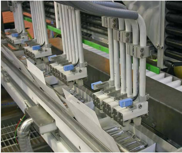
Robotics Can Be Offered as Option Modules or Integral to the Machine, as in this Display Carton Packer from Cavanna
