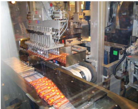
This Somic Cartoner Is Essentially a Cluster of Robotic Arms and Servo Collating Belts. Introduced at Interpack These Machines Have Already Been Installed in the U.S. and Canada
