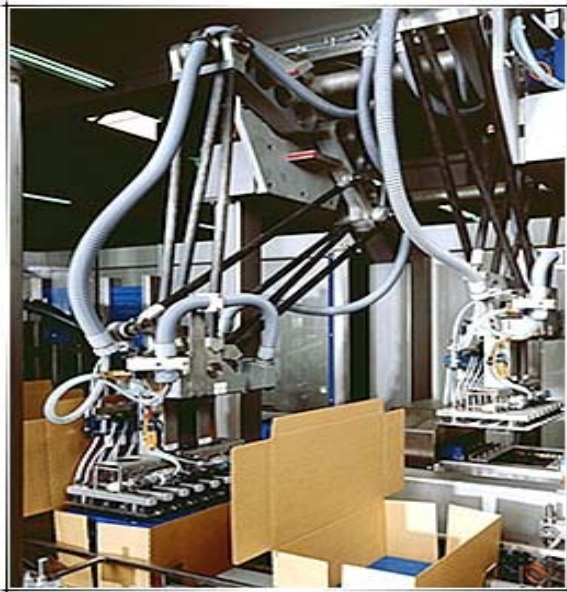
A+F Robotic Case Packer with Graphite Arms Combines Speed and Payload Capacity
